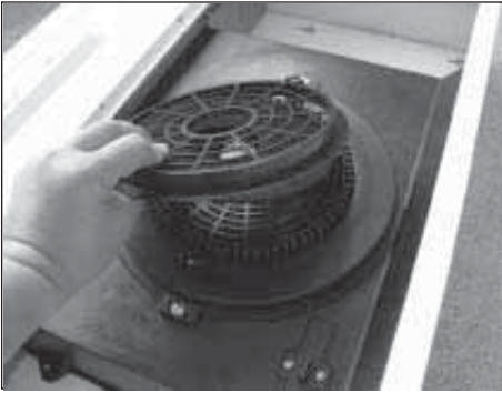
2. Remove the carbon filter and carbon filter holder.
